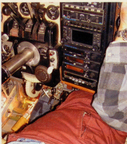
One of the more agonizing tasks was replacing all of the engine control cables. The cables are fed into the fuselage (below) and attached to the appropriate control lever behind the panel (left).
