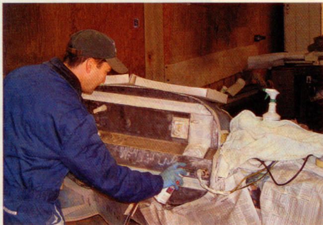
After being completely stripped of 36 years of grime, the firewalls were primed and painted white (above). After several hours of flight time, Dave Hopkins and the brothers check on the engine's status (right).
