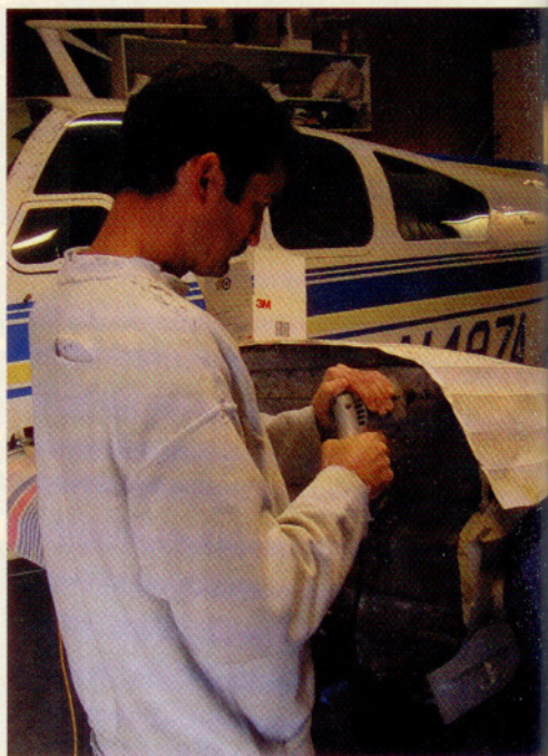
Rob Bedell strips the firewalls to bare metal—another labor-intensive task.
